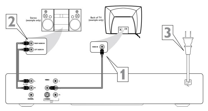
Connect the supplied video cable to the yellow VIDEO (VIDEO OUT) jack of the Player and to the TV's VIDEO IN jack. The supplied video cable has yellow ends.
